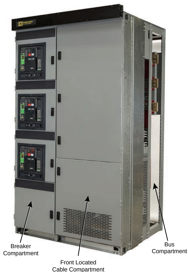
Typical Power-Zone 4 Front Accessible Switchgear Section (42" deep)
