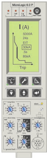
Figure 29 - Type P (Power Metering) Trip Unit
