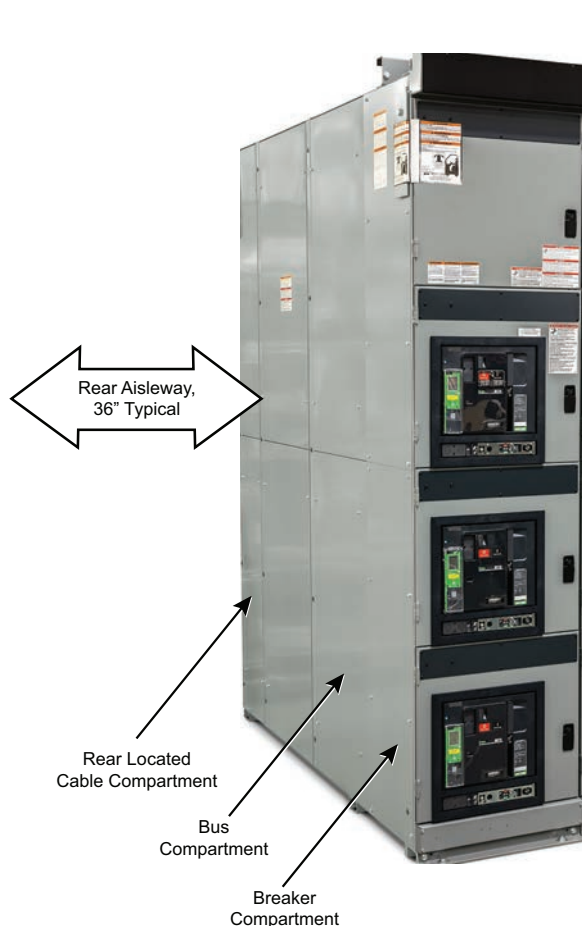
Typical Power-Zone 4 Rear Accessible Switchgear Section (72 – 80" deep)
