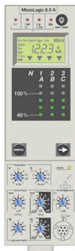
Figure 28 - MicroLogic Type A (Ammeter) Trip Unit
