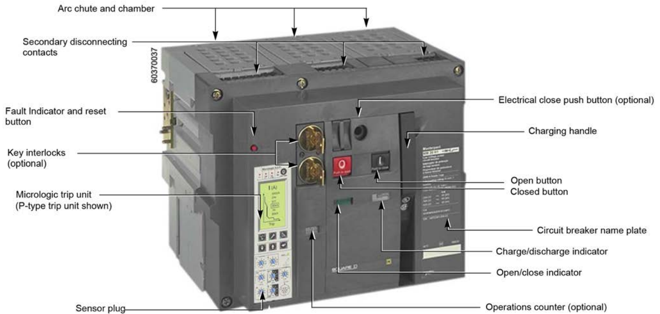
Figure 21 - Typical MasterPacT Circuit Breaker (Front and Side View of NW shown; MTZ is similar)
