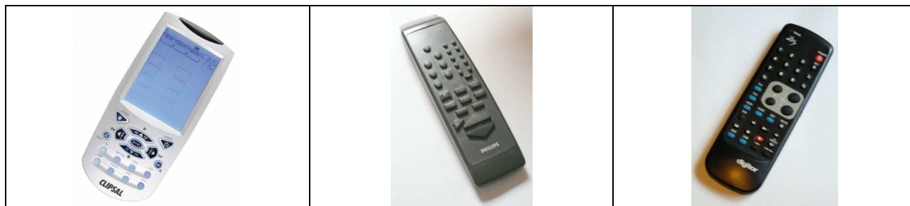
Typical generic IR remotes with on-board NEC codes
