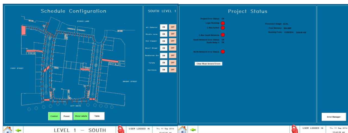
Figure 4: Sample Schedule Plus layouts showing an example of Lighting Control status information available at the Building Layer
