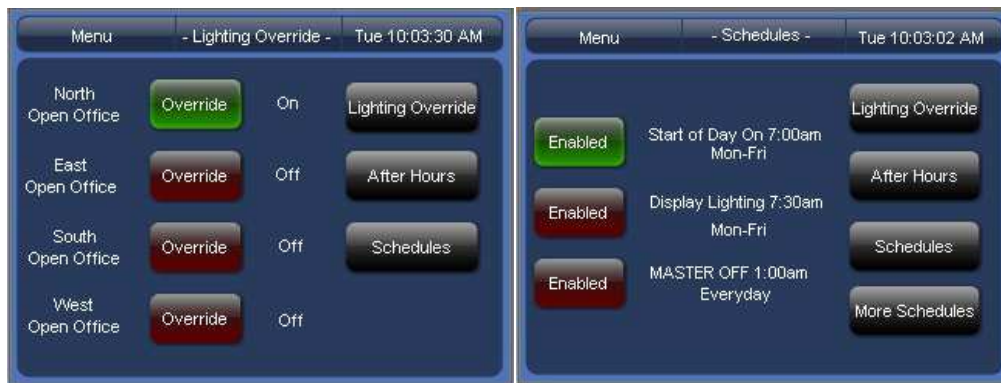
Figure 2; Sample Touchscreen layouts showing an example of Lighting Control status information
