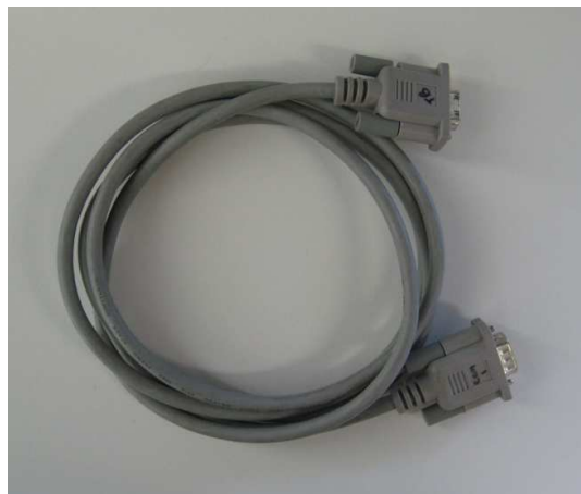
Figure 3 – DB9 Male to DB9 Female Extension Cable
