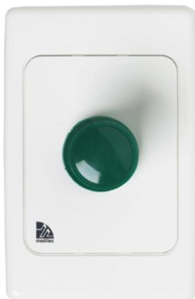
The Equipotential Junctions shall be the ESP Series catalogue no. E34 or E35 and shall comprise of a fully insulated green screw clamp terminal with a terminal head size of 26mm in diameter labelled “EQUIPOTENTIAL JUNCTION” and a buss bar with line tap (E34 – 5 x 5mm tunnels, E35 – 10 x 5mm tunnels & 4 x 8mm tunnels).
