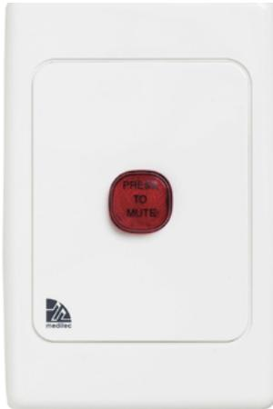
Each RCD shall have an Audible Alarm to highlight that the RCD has tripped. The Audible Alarms shall be the Clipsal ML2000 Series catalogue no. ML2031E08 Series and shall comprise of a mutable two tone audible alarm, flashing red visual alarm, and mute push button labelled “press to mute”
