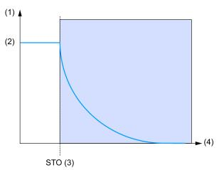
(1) Motor speed - (2) Actual speed - (3)  $\overline{\text{STOA}}$  and  $\overline{\text{STOB}}$  - STO Activation - (4) Time
