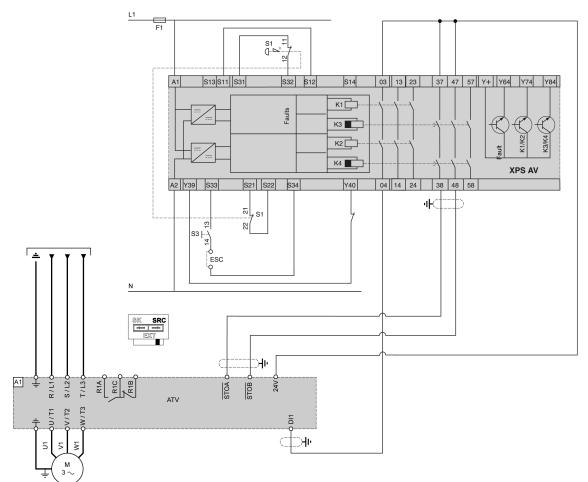
**NOTE:** This diagram is a wiring configuration using DI1 assigned to forward operation.
