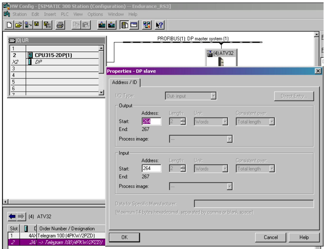
By default, the process data are linked to **(C P d)**, **(L F r d)**, **(E E R)** and **(r F r d)** (native CiA402 profile of the drive). You can check that the exchanges are working properly by the Monitor / Modify function of the configuration tool:
