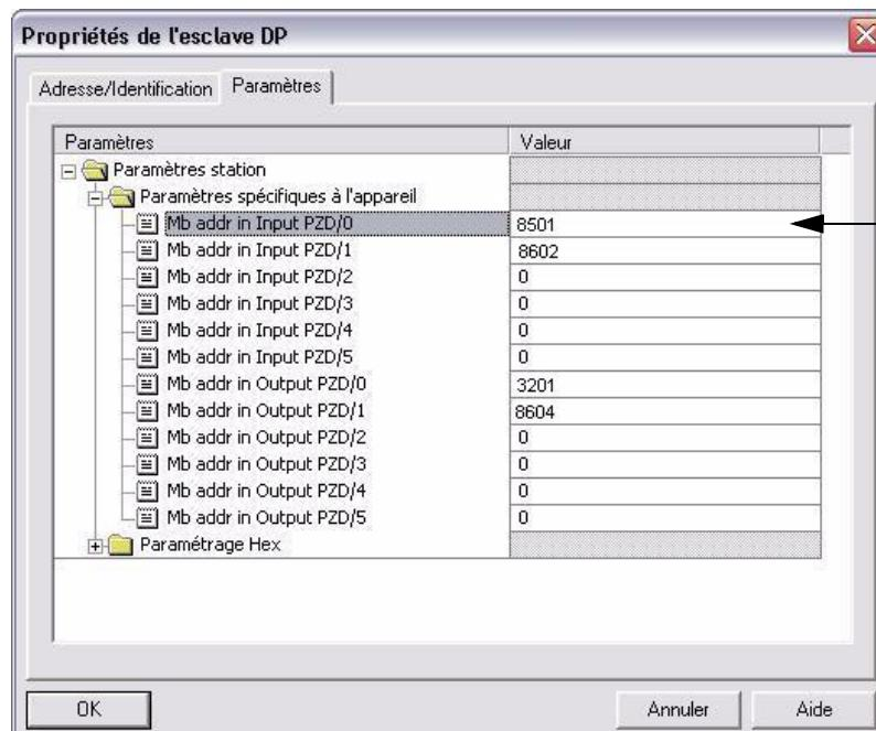
When the exchanges are performed (PROFIBUS network is running) you can check the configured parameters by reading from the ATV32 HMI the configured Modbus address: with the (**D C R x**) and (**D P R x**) parameter in the PROFIBUS option menu of the drive.
