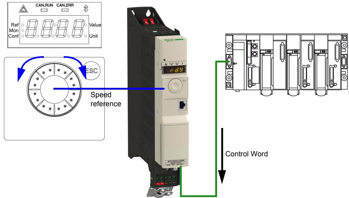
The drive is controlled from the communication (1 of the 3 following settings MDB, CAN or NET) but the reference is adjusted on local HMI. The control word comes from the controller and is written according to CiA402 profile.
