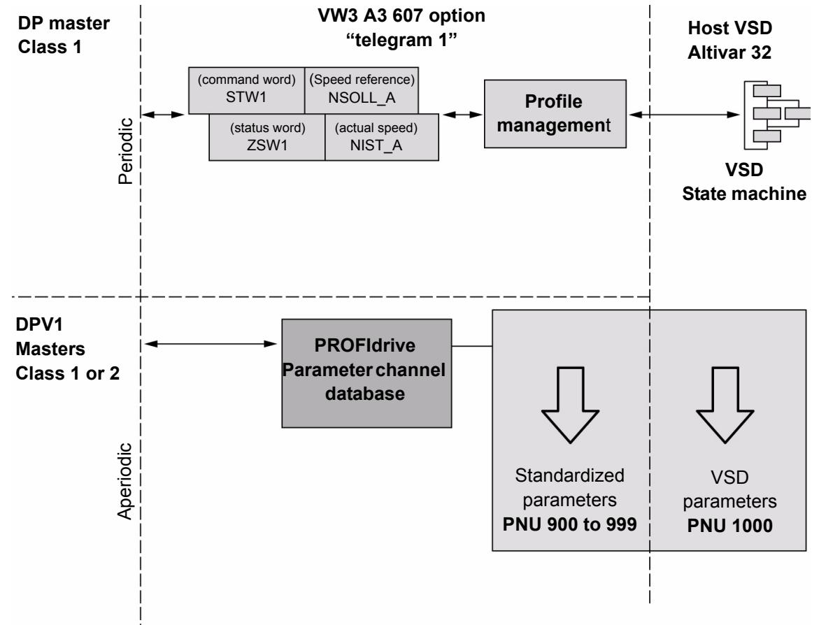
The Altivar 32 is controlled with the process data (PPO3) by a DPV0 or DPV1 master. The command and status process data are compliant with IEC 61800-7/PROFIdrive.
