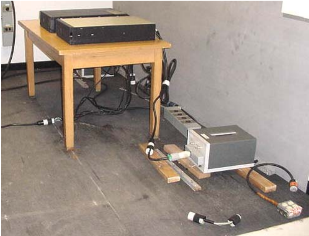
Configuration for Conducted Emissions
