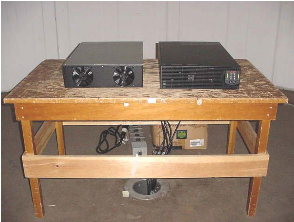
Configuration for Radiated Emissions (Front)
