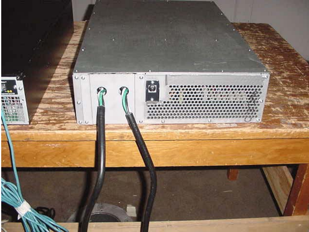
Configuration for Radiated Emissions (Rear Closeup)
